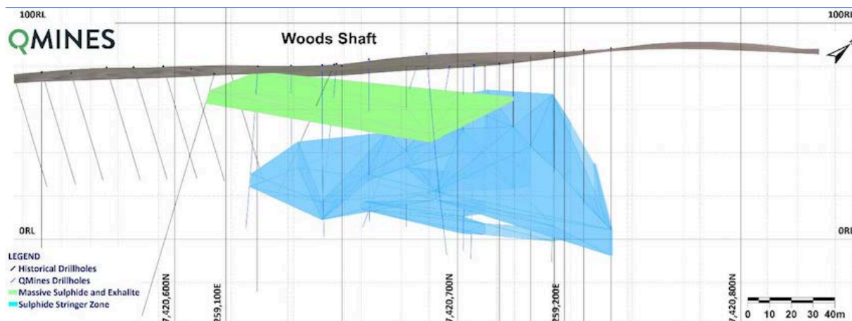
Figure 20: Woods Shaft Resource showing the Stringer and Massive Sulphide zones
